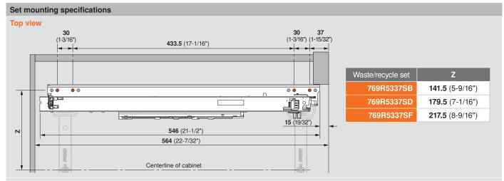
NOTE: Orange dots indicate pre-mounted screw locations. All four are required to meet specified load capacities.
