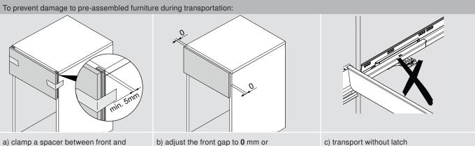
a) clamp a spacer between front and cabinet or
