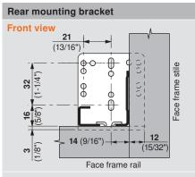
**NOTE:** For frame applications, use a minimum of three screws per bracket
