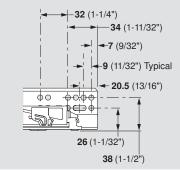
**NOTE:** Elongated holes are for  $\pm$ **4.5** (3/16") depth adjustment only. Additional screws must be used to secure the runner to the cabinet.
