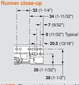
**NOTE:** Elongated holes are for  $\pm$ **4.5** (3/16") depth adjustment only. Additional screws must be used to secure the runner to the cabinet.
