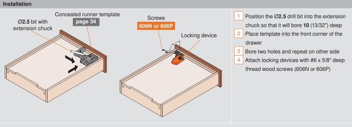
**NOTE:** The mounting screws must go in at a precise angle and the locking device must fit flush to the drawer bottom to ensure proper function of the complete drawer system
