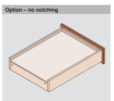
Make the back panel shorter and extend the drawer bottom to the back of the drawer
