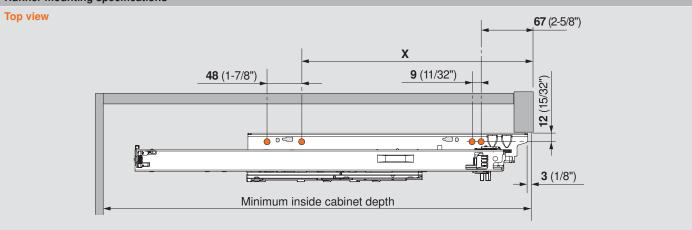
NOTE: If using 15/32" or 1/2" drawer thickness without T59.K010M, subtract 3 (1/8") from setback and screw locations.
