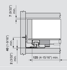
**NOTE:** MOVENTO runners will sit **2** (3/32") higher when using the lateral stabilizer in bottom mount applications and may have to be raised for some bottom mount drawer applications using SERVO-DRIVE
