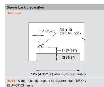
Do not use bumpers, as this can inhibit the function of TIP-ON BLUMOTION when the drawer front is pressed.
