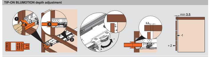
**NOTE:** Using the 65.5632.US front gap template is highly recommended. Adjust left and right runner.
