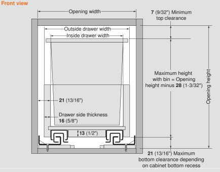
NOTE: Drawer side material thickness may vary. Precise measurement of drawer side material thickness should be used when calculating outside drawer width using the table below. Inside drawer width **must** equal opening width minus **42** (1-21/32") for MOVENTO runners to align and function optimally.
