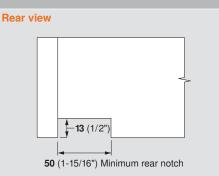
The notches must be flush with the drawer sides and bottom
