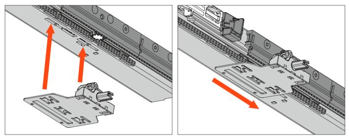
Fitting the driver pins to the runners
