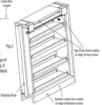
**Step 2.** Install upper and lower scribe rails to filler pullouts being careful not to split the wood. If using screws to attach, be sure to pre-drill first. Align scribe rails with front edge of filler pullouts. Align scribe rail to upper section of base cabinet lower mounting. (See Fig 2) **Note:** If installing pullout in a frameless application, it is recommended to that a 1/16" thick scribe rail be used to space the filler unit properly.
