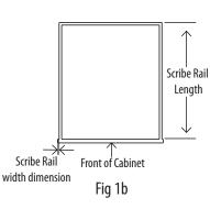
**Step 1**. Measure scribe rail thickness and length per your specific cabinetry. (See Fig 1a and 1b)
