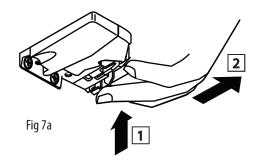
**Step 1**. Press up on adjustment tab.
