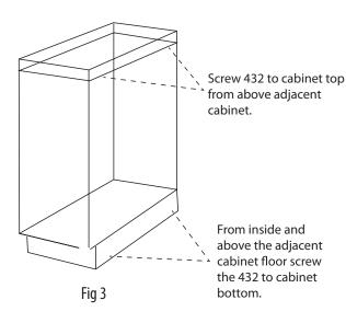
**Step 3.** Pre-drill holes using your 3/16" drill bit. See the table below for measurements specific to your filler height. After pre-drilling has been completed on one cabinet side, repeat with adjacent cabinet.
