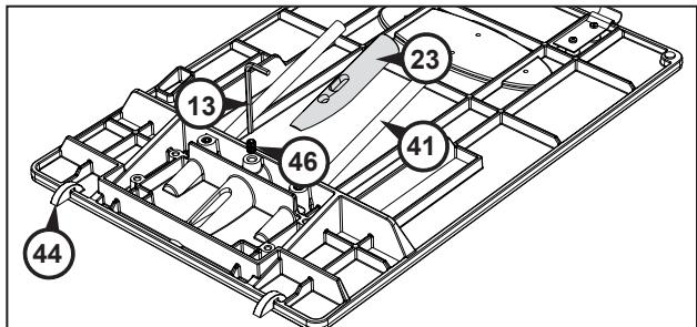
Place the access panel upside down on a flat surface (for example, a tablesaw table). Loosen the drill-guide set screw (46) with the 3mm hex wrench (13) and remove the drill guide. Firmly holding the access cover against the flat surface, slide the new drill guide into the opening, rotate it so the angled face is against the flat surface, and tighten the set screw.
