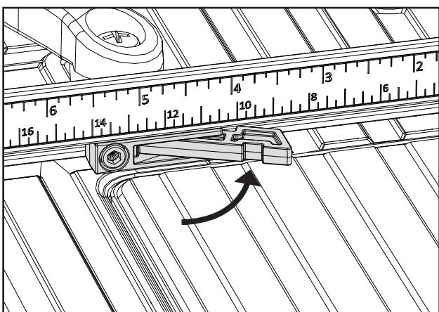
Each stop arm can be held in the retracted position by pressing the arm into the stop body and then sliding it toward the socket-head bolt that secures the stop in the fence. The notch in the arm provides a grip point. To reactivate the stop arm, slide it away from the bolt.
